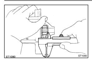
(b) Move the pinion gear toward the stop collar to remove slack and measure the clearance between the pinion gear end and starter housing.
