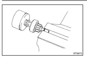
(c) Apply grease to the snap ring, and install it to the planetary carrier shaft groove.
