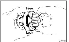
Check the starter clutch. (b) Rotate the clutch pinion gear clockwise and check that it turns freely. Try to rotate the clutch pinion gear counter-
