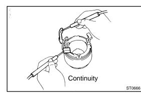
7. INSPECT FIELD FRAME (FIELD COIL) FOR OPEN CIR-CUIT
