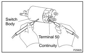
(c) Check the hold-in coil for open circuit. Using an ohmmeter, check that there is continuity between terminal 50 and the switch body.
