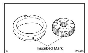
If it is more than the maximum, replace the vane plate and/or vane pump rotor with the one having the same mark stamped on the cam ring.
