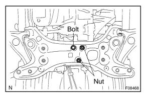
11. DISCONNECT ENGINE REAR MOUNT INSULATOR AND FRONT SUSPENSION MEMBER
