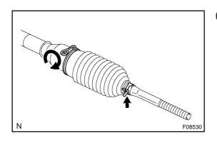
(b) After winding and tightening the clamp around the circumference of the boot twice, twist it several times, and install it.
