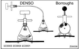
(b) Using a belt tension gauge, measure the belt tension. Belt tension gauge: DENSO BTG-20 (95506-00020) or Borroughs No. BT-33-73F Drive belt tension: New belt: 440 - 540 N (45 - 55 kgf) Used belt: 240 - 340 N (25 - 35 kgf)
