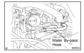
(b) Connect the 2 water bypass hoses to the throttle body.
