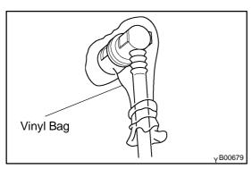
(e) Prevent the disconnected fuel tube from damaging and mixing foreign objects by covering them with a vinyl bag.
