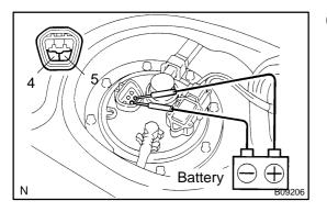
(e) If you have no TOYOTA hand-held tester, connect the positive (+) lead from the battery to terminal 4 of the connecter, and the negative (-) lead to terminal 5.
