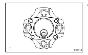
(b) Place the ABS speed sensor on the axle hub so that the connector is set at the bottom under the on-vehicle condition.
