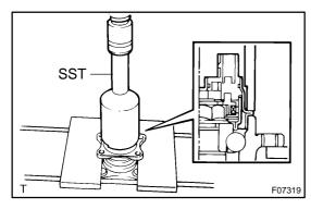
(c) Using SST and a press, install a new ABS speed sensor to the axle hub.
