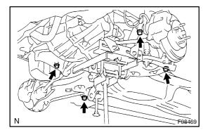
(b) Remove the 4 bolts and lower the suspension member.
