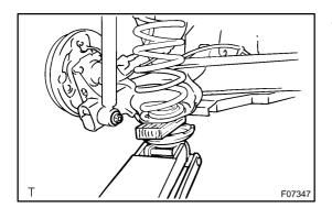
8. SUPPORT REAR AXLE BEAM AT RIGHT AND LEFT SIDES WITH JACKS
