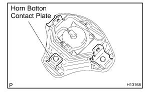
Check the deformation on the horn button contact plate of the steering wheel pad.
