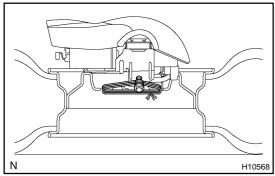
(3) Face the upper surface of the steering wheel pad upward. Separately tie the left and right sides of the steering wheel pad to the disc wheel through the hub nut holes. Position the steering wheel pad connector so that it hangs downward through a hub hole in the disc wheel.
