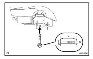
(1) Install the 2 bolts with washers in the 2 bolt holes in the steering wheel pad.
