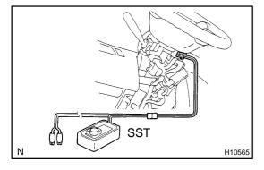
(3) Connect the connectors of the 2 SST to the airbag connector of the spiral cable back side.
