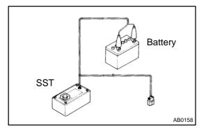
Connect the SST to the battery.
