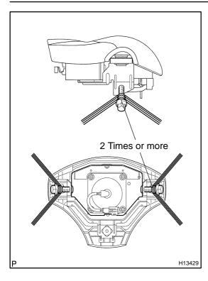
(2) Using 3 wire harness, wind the wire harness at least 2 times each around the bolts installed on the left and right sides of the steering wheel pad.
