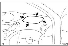
• There should be no interference between the instrument panel and the front passenger airbag assembly.
