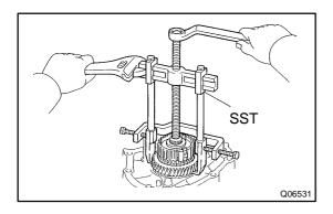
(b) Using SST, remove the No. 3 clutch hub assembly, 5th gear and synchronizer ring.
