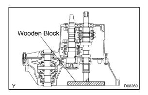
Before driving in the No. 3 clutch hub assembly, place the suitable sized wooden block on the rear side of the input shaft, as shown in the illustration. When driving it in, fix the input shaft firmly so that it is not pushed downward. Otherwise the input shaft rear bearing is overloaded, it might be damaged.
