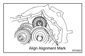
Install the reverse idler gear, thrust washer and shaft, as shown.
