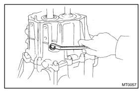
17. REMOVE REVERSE IDLER GEAR SHAFT LOCK BOLT AND GASKET
