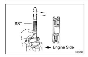
Using SST and a hammer, drive in the No. 3 hub sleeve assembly with the No. 3 shift fork.
