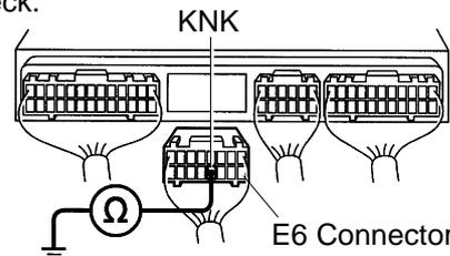
Connector being checked is disconnected.
