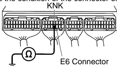
Connector being checked is connected.
