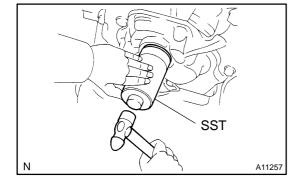
(c) Using SST and a hammer, tap in the oil seal until its surface is flush with the timing chain cover edge.
