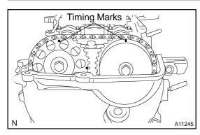
(b) Check that both timing marks on the camshaft timing sprocket and valve timing controller assembly are facing right up as shown in the illustration.
