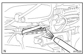
Using a timing light, check the ignition timing.
