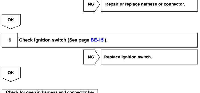
Check for open in harness and connector between IG switch and EFI relay and body ground (See page IN-29).
