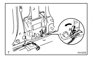
(c) Disconnect the pretensioner connector as shown in the illustration.
