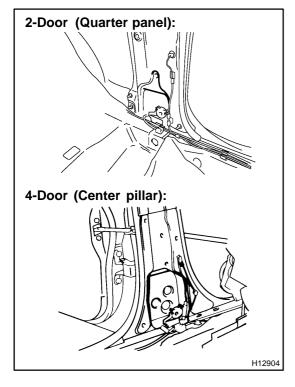
• Check for cuts and minute cracks in wire harness or marked discoloration on the front seat outer belt.
