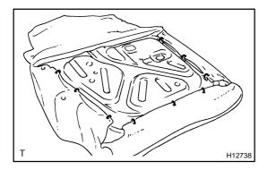
(c) Install the hog rings as shown in the illustration. HINT:
