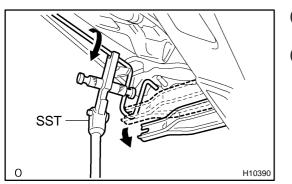
(b) Install SST to the torsion bar on the hinge side. SST 09804-24010
