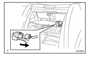
(b) Remove the connector cover from the lower instrument panel.
