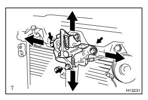
3. ADJUST HOOD LOCK Adjust the lock by loosening the 3 bolts. Torque: 7.8 N-m (80 kgf-cm, 69 in.-lbf)
