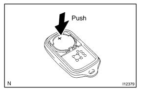
(c) Remove the battery (lithium battery) as shown in the illustration.
