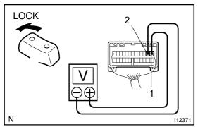
(c) Reverse the polarity of the voltmeter leads.
