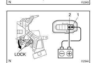
(b) Reverse the polarity and check that the door lock link moves to LOCK position.
