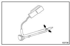
(d) Release the 2 claws and remove the thermistor from bracket plate.
