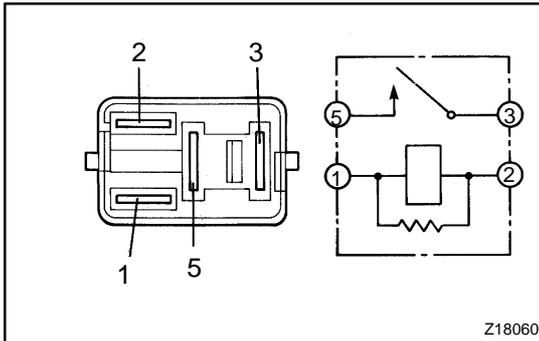
2. INSPECT MAGNETIC CLUTCH RELAY (Marking: A/C MG) CONTINUITY
