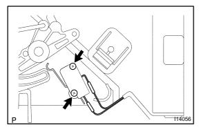
5. Two way flow heater models only: REMOVE MICRO SWITCH (for MAX. WARM)
