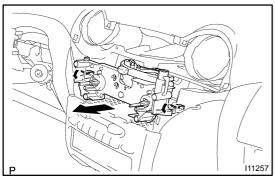
6. REMOVE HEATER CONTROL ASSEMBLY
