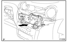
(c) Fit the 2 claws of heater control assembly in the instrument panel hole.
