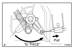
(f) Adjust defroster control cable. Pull the air inlet control link to "FACE" position, connect the control cable and lock the clamp.
