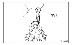
(c) Using SST, remove the snap ring. SST 95994-10020
