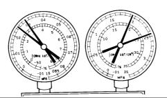
NOTE: These gauge indications are shown when the refrigeration system has been opens and the refrigerant charged without vacuum purging.
