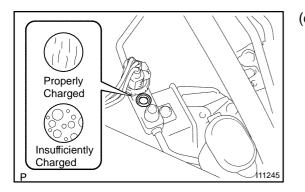
(d) Charge refrigerant until bubbles disappear and check the pressure on the gauge through the sight glass.
